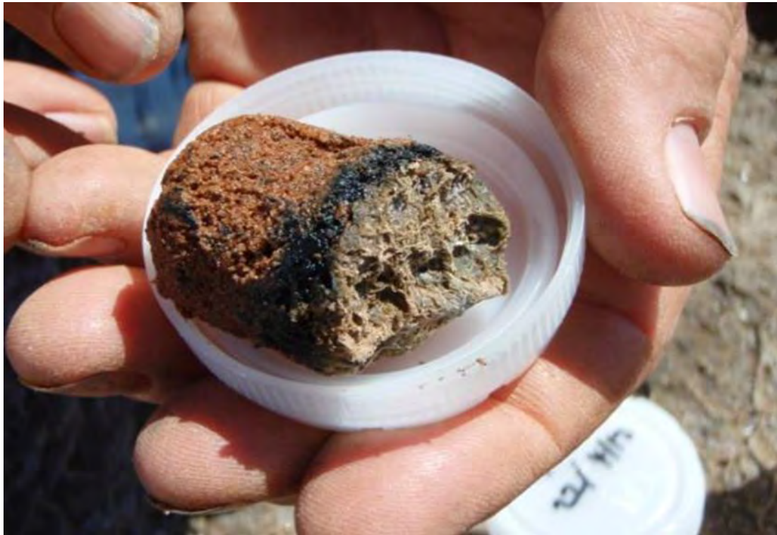
Figure 6-25 Typical core sampled from an algal mat area showing a thin veneer (~5 mm thick) of algal mat and under-lying sediment
